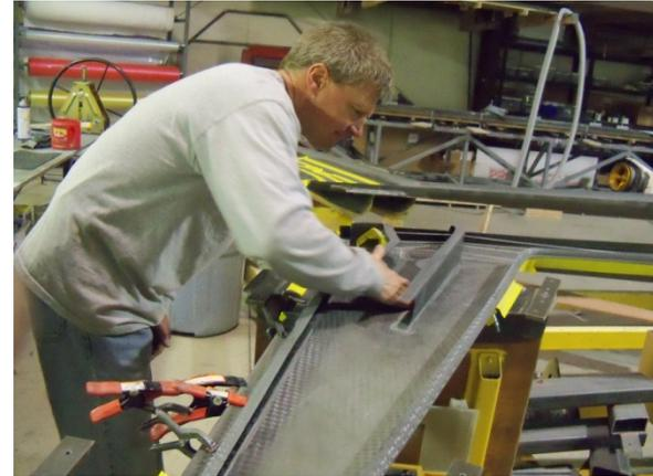
Factory assistance (optional) is available for closing the wings, horizontal, and fuselage in the factory jigs. Drawings are provided for those that wish to construct their own jigs and fixtures for the assembly of these components.
