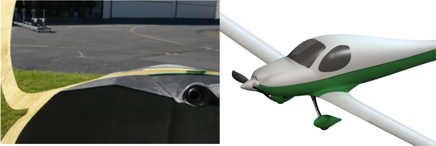
Pilot comfort is a very important part of the equation in an aircraft designed for long soaring flights. The cabin features side by side seating (practically no CG change with loading) with excellent field of view. A large instrument panel designed for modern screens is placed within easy reach. Powerful cabin ventilation is designed in as well as ergonomic seating and built in provisions for oxygen and baggage storage are additional niceties.
