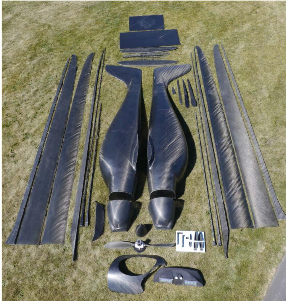
This is a composite aircraft kit. It includes the molded oven cured composite parts that can not be reproduced without the molds. Composite flat panels are provided for fabrication of certain internals. Drawings are provided for these shapes as well as for the metallic parts. Fabrication of these parts requires basic skills such as cutting, drilling, riveting, bending, and welding.
